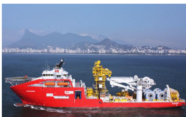
Figura 1 – Pipeline layer support vessel
